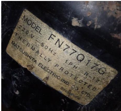
Figure 5: Refrigerator nameplate on a compressor
