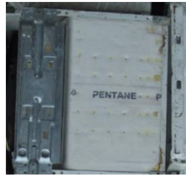
Figure 6: Refrigerators containing pentane will not be relevant for carbon credits. Here the backside indicates pentane
