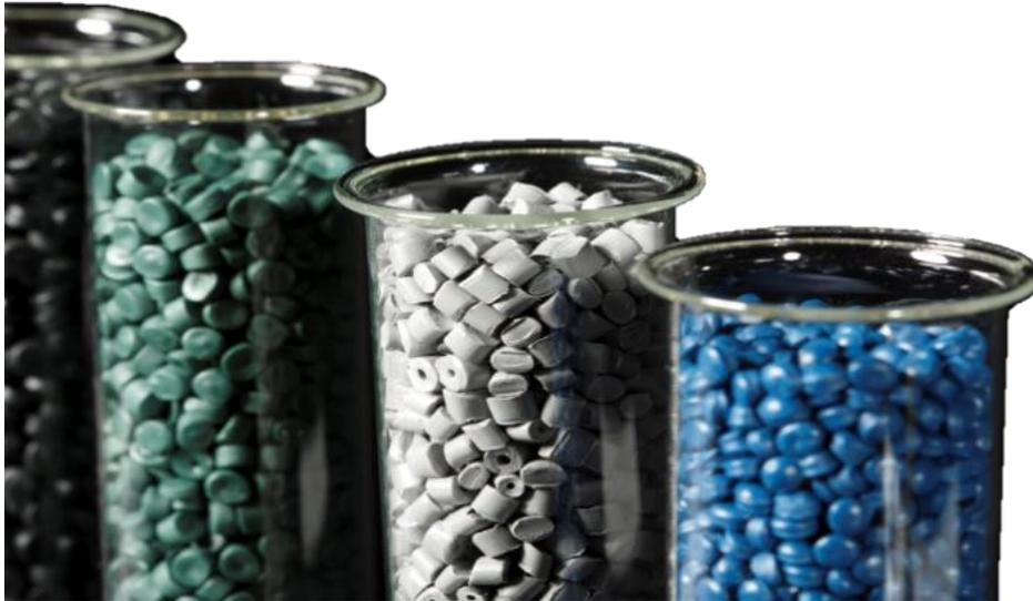
Photo 2: PE regranulates (© Vogt-Plastic GmbH 2020)
